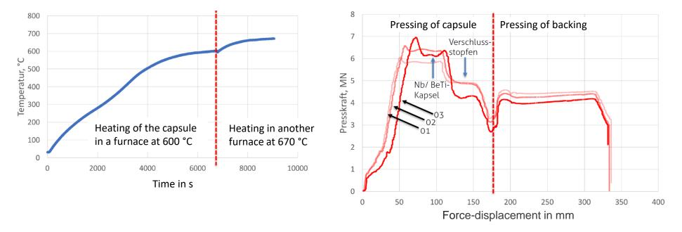
Increasing Be-Ti fraction leads to an increasing pressing force and the decreasing off the stationary press area (reason: increasing compaction energy)
